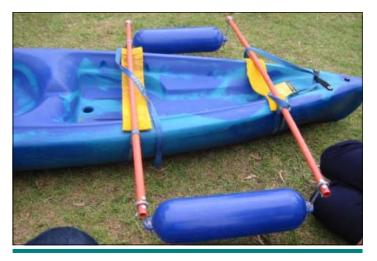
Designed by CV staff, these outriggers have proved successful in the All Abilities canoeing program...
